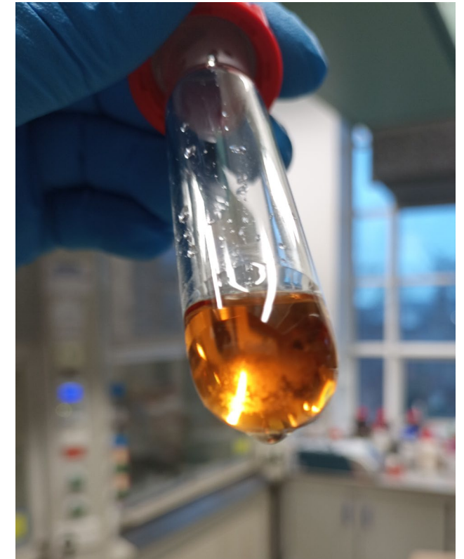
Fig.7 Nd acetate crystals precipitate in BMIM acetate
